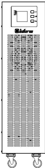
Fig.1 6/10kVA(S) Front Panel view
