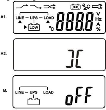
3.13.1.5 Then, the UPS is on Bypass Mode now and it will proceed self-test automatically. If there is no abnormal message occurred, it means the prestartup of the UPS is successful and the charger starts to charge the batteries.
