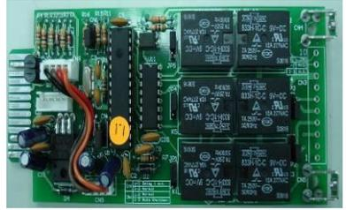
6.5.2 The shutdown function will be activated, after a +6~-+25Vdc is put between pin9 and pin10 for 5 seconds.
