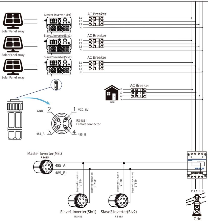
Pic 7.27 CHINT Connection diagram(The pass-through table)
