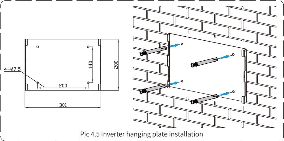
Pic 4.5 Inverter hanging plate installation
